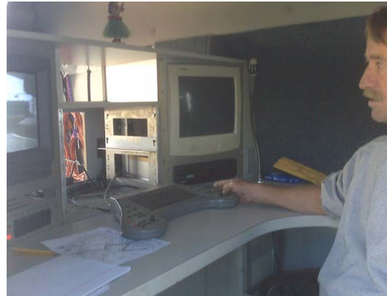
Viewing camera feed from sewer line
